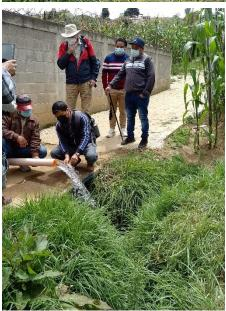
Well/pump flowrate measurement and water sampling
